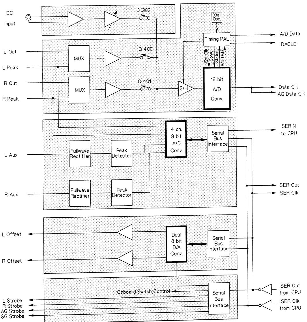
Fig. 11.1 - A/D Converter Block Diagram
