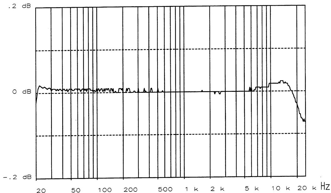
Fig. 17.4 - Audio Generator Ripple, Typical
