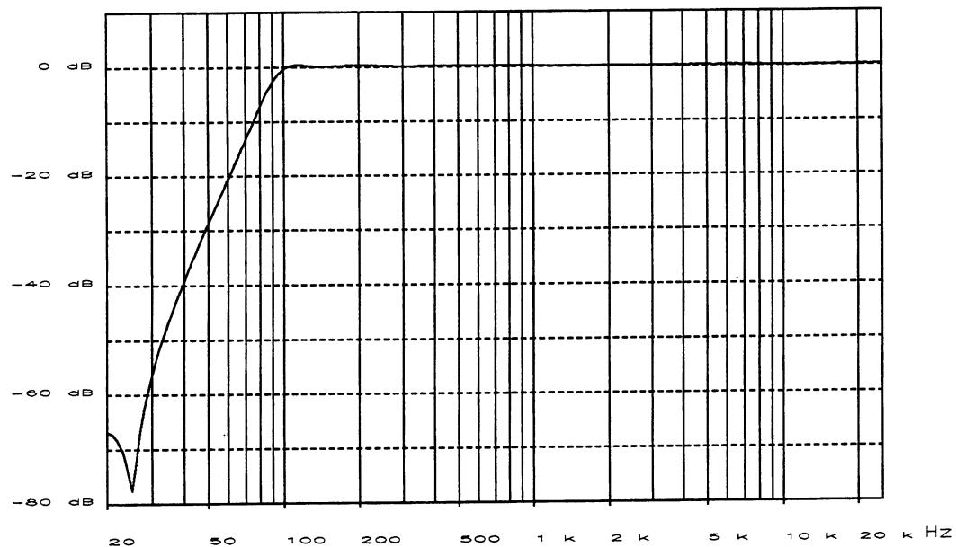
Fig. 17.14 - 100 Hz High-pass with 25 Hz Notch
