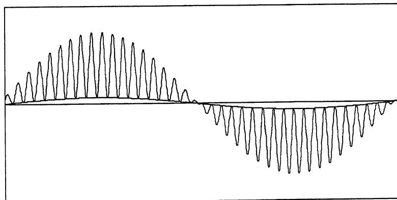
Fig. 13.2 - Adjustment of LR Separation
