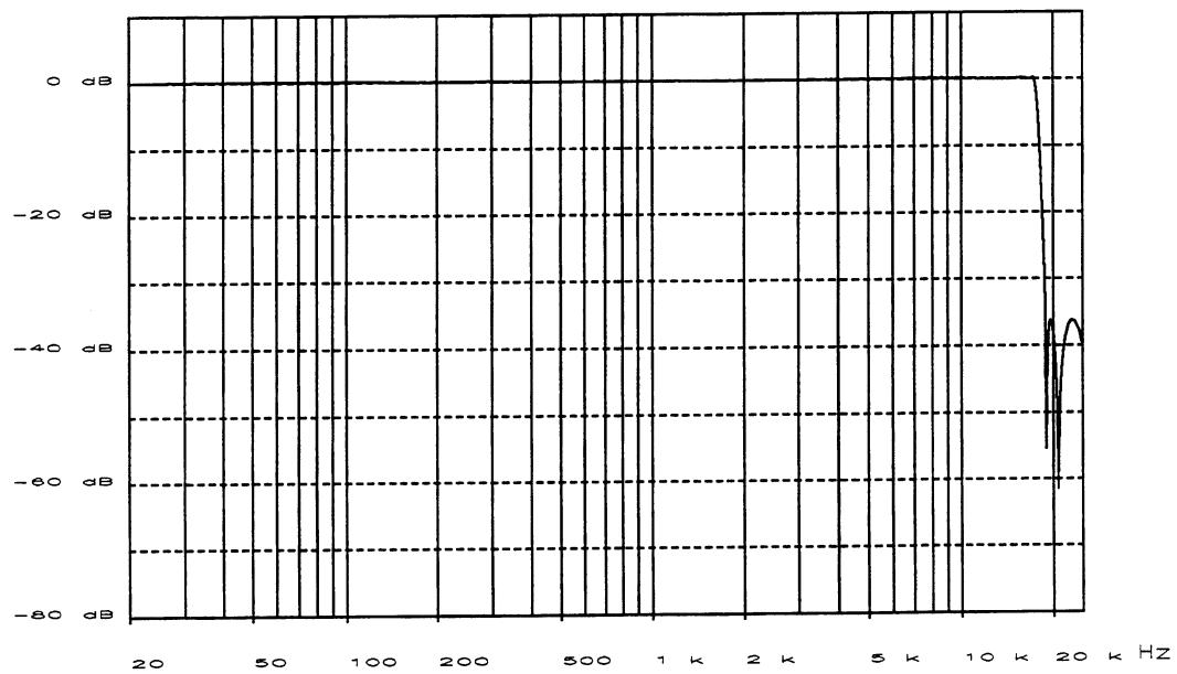
Fig. 17.11 - 15 kHz Low-pass with 19 kHz Notch
