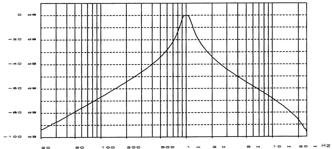
Fig. 17.18 - Double Precision Band-pass, 1 kHz
