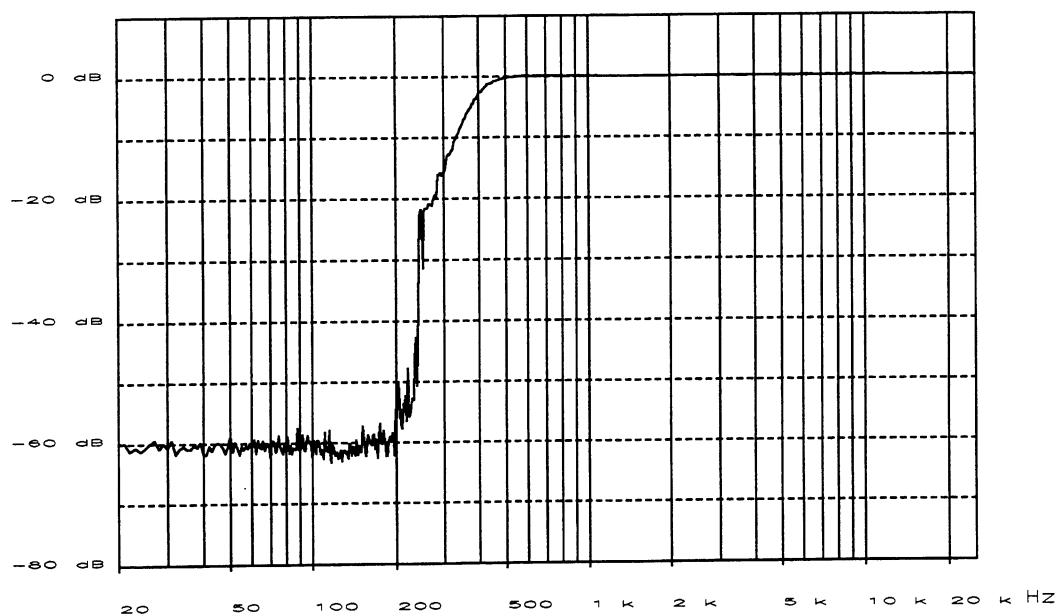
Fig. 17.16 - 400 Hz High-pass
