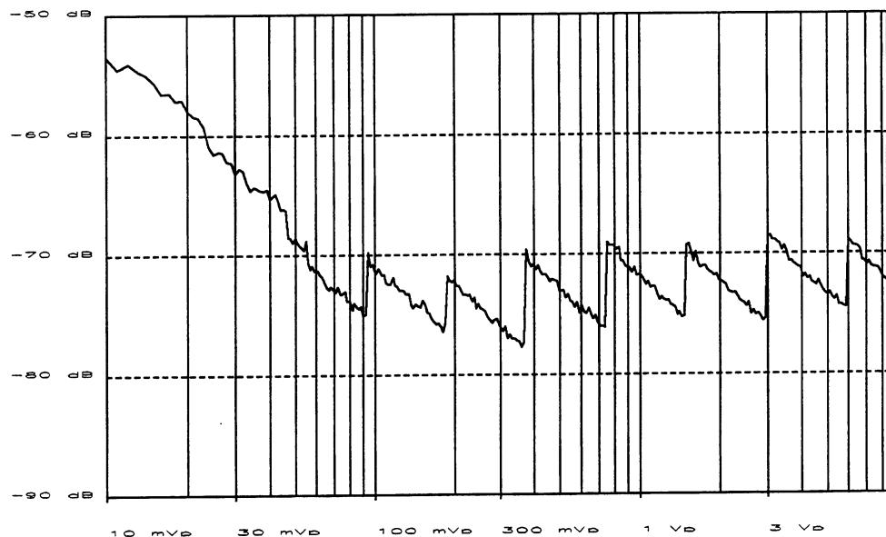
Fig. 17.3 - SINAD versus Level, Typical,
