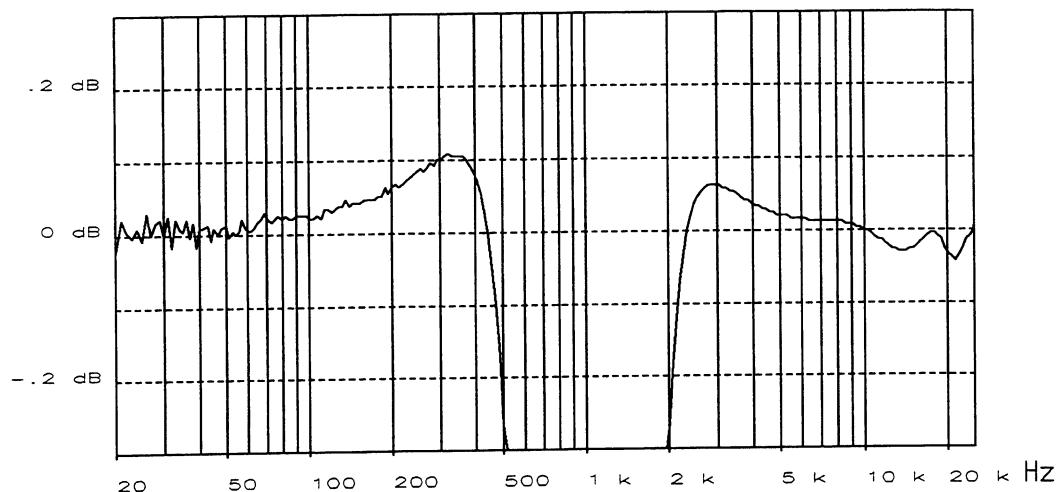
Fig. 17.20 - Notch Filter Ripple
