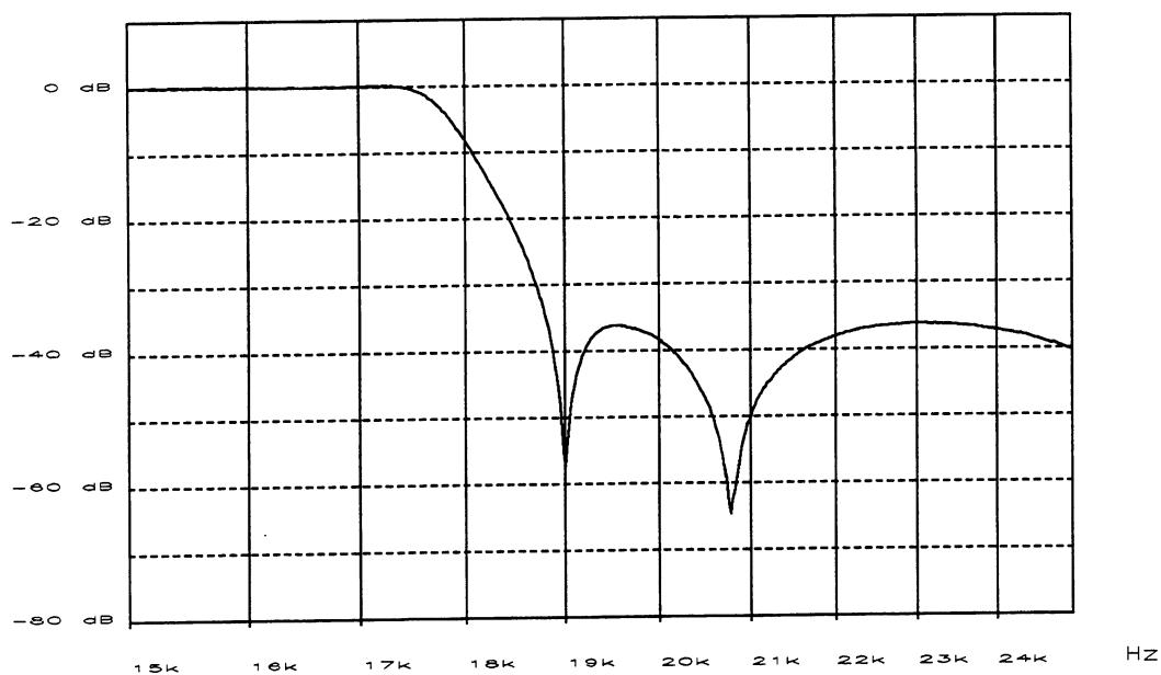
Fig. 17.12 - 15 kHz Low-pass, Stopband Characteristic
