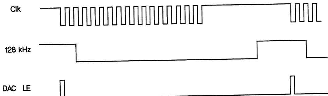
Fig. 12.1 - A/D Converter and Audio Generator Timing
