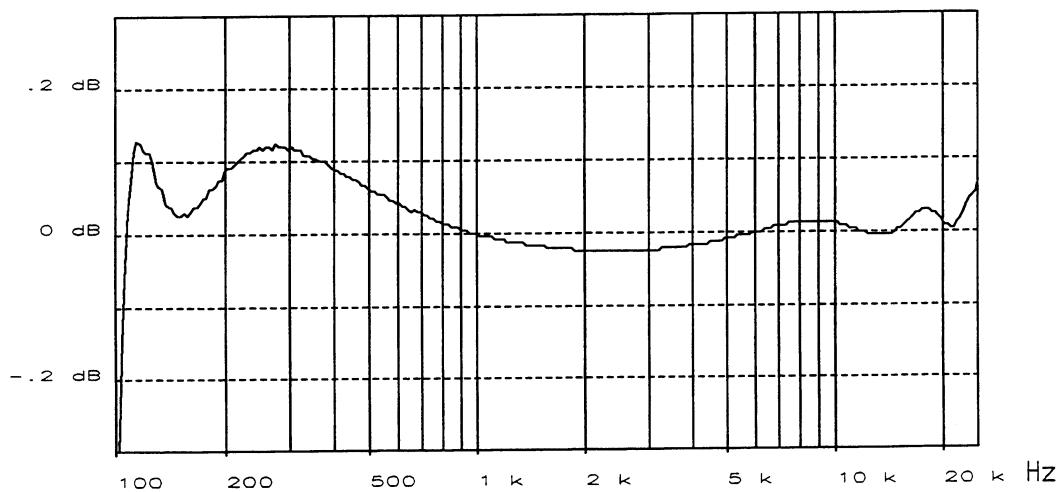
Fig. 17.15 - 100 Hz High-pass Ripple
