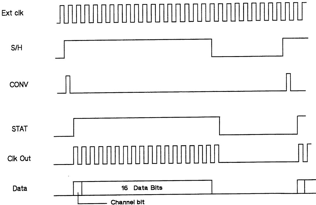
Fig. 11.2 - A/D Converter Timing
