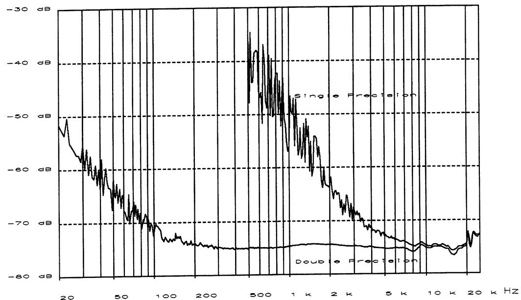
Fig. 17.21 - Notch Filter Attenuation at Notch Frequency
