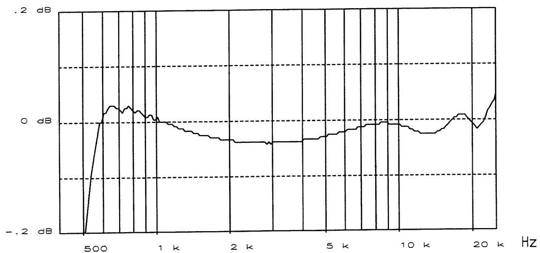
Fig. 17.17 - 400 Hz High-pass Ripple
