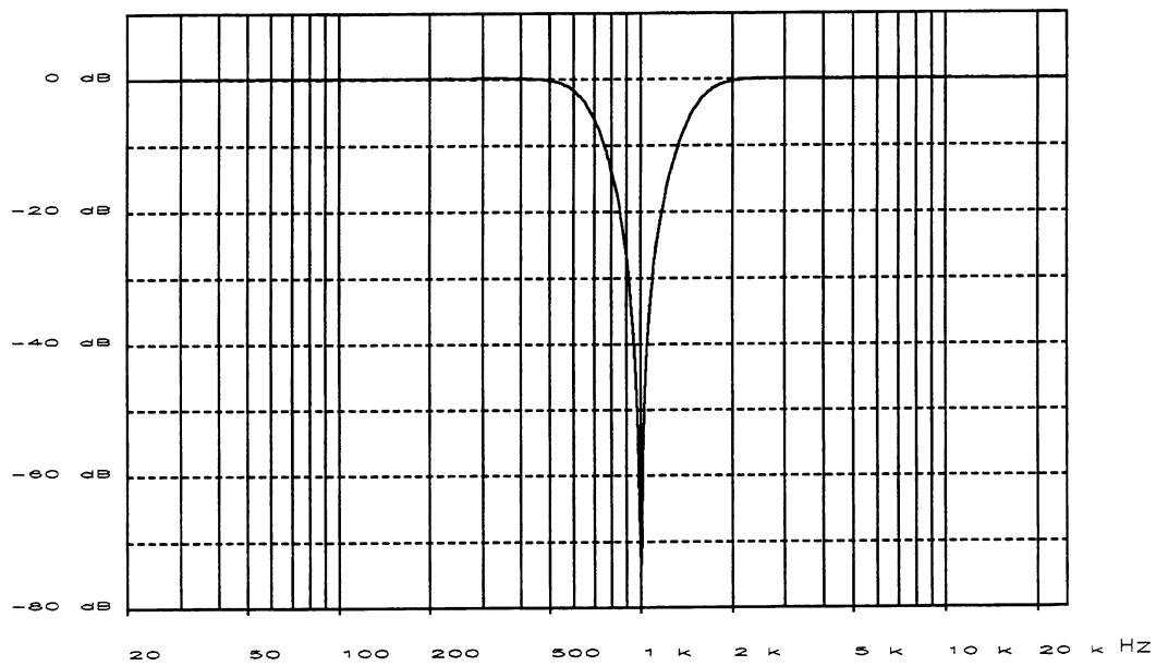
Fig. 17.19 - Notch Filter, 1 kHz
